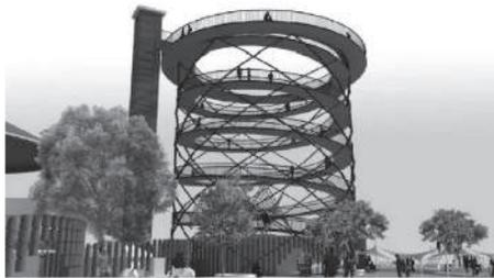
The grid-like/akin steel structural members of the Tower are, according to the firm, inspired from the bird's nest. It is further expected to give 'a sensational and dramatic effect' to the visitor as the structural members are woven and inter-woven around the ramp. One other feature of the Tower is that maximum space is provided in the deck area so that visitors could 'enjoy the grand view from the top'.
